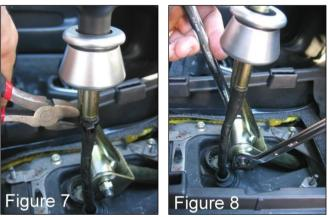
7. Use the circlip (or needle-nose) pliers to remove the circlip retaining the gearstick ball cup (fig. 9). Pull up on the gearstick as you close the circlip, it should lift out once the circlip clears its groove. Pull the reverse lock cable out of the gearstick as you lift it out.
